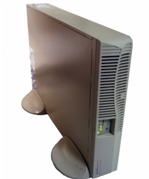
Illustration 2-11: 3 kVA UPS - model 9130
